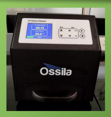
Application: To change the surface properties from hydrophobic to hydrophilic.
