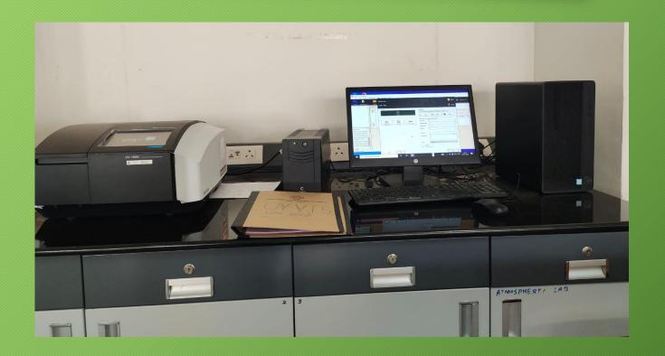
Application: Absorption spectrum of thin film and liquid in Uv-vis range
