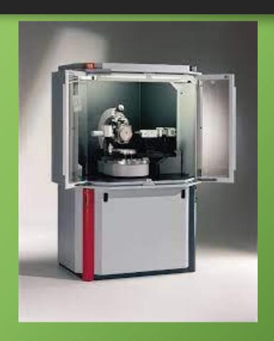
Application: To determine the crystal orientation in thin film and powder samples.
